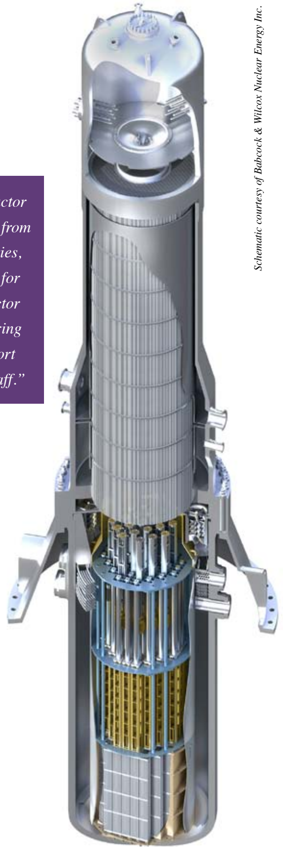
Babcock & Wilcox mPower™ small modular reactor schematic.
